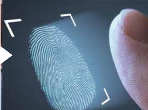
BCI/AFIS has a newly implemented 2-finger rapid ID search. This technology can take an individual's right two fingerprints on a scanner and search a database to see if the individual has previously been fingerprinted in RI. If found, previous fingerprints can be resent for the national background check to the FBI for processing, significantly expediting the transaction.
